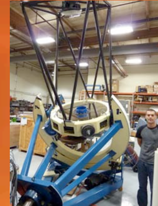
April 2010, first complete 1m in shop. Mirror cell with primary location clips, ports for cables, fans and embedded control blackfins & bolt circle for instrument. The telescope is being commissioned with a 4K SBIG CCD with internal guider. The science Fairchild CCD486, with in-house Sinistro controller, 2 off-axis guiders, fiber feed for MedRes Spectrograph and fast photometry port will be commissioned in 2011.
