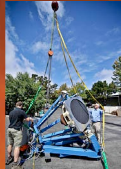
The complete, aligned mount, mirror cell, with primary installed, cover, temporary (0.4m) control panel.
