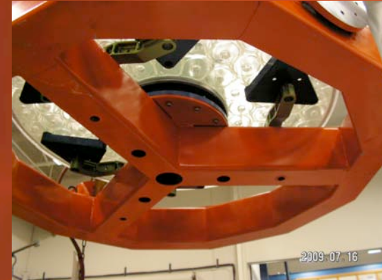
July 2009. Test fixture illustrates 18-pt whiffle for axial support, and central hub contacting via O-rings on upper & lower inner diameters of the Hextek primary. M1 tilt is \pm 35 \mu at edges, radial \pm 20 \mu , no hysteresis. Mirrors were polished, coated (and SiO2 overcoated) at LZOS, Russia.
