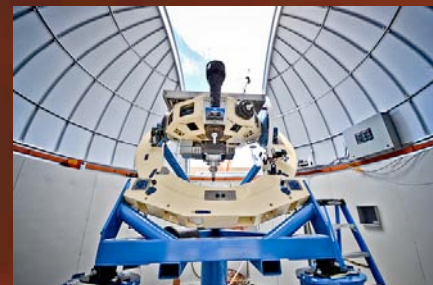
Primary is 2m above grade level. Piers are on isolated concrete. Lens/CCD are for quick mount alignment and "Context" imaging. A collimating telescope is mounted temporarily at the Cassegrain.
