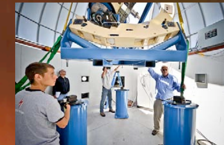
Mount lowered onto fixators on piers for easy polar alignment.
